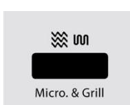
In this operating mode, the device works in microwave mode for 30% of the cooking time and in grill mode for 70% of the cooking time.
