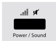
Press the button **Power/sound** for three seconds in order to switch on or off the sound (beep tone).
